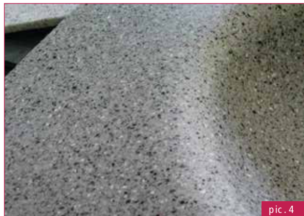
pic.4 2D small radius with whitening effect by darker colour
