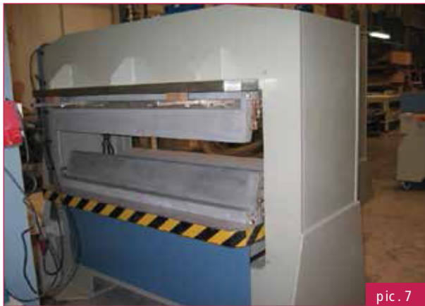
pic.7 Global press & alu cooled mould
