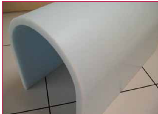
pic. Shows a thermoformed S303 R = 85
