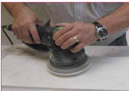
Sanding with a random orbital hand sanding machine
